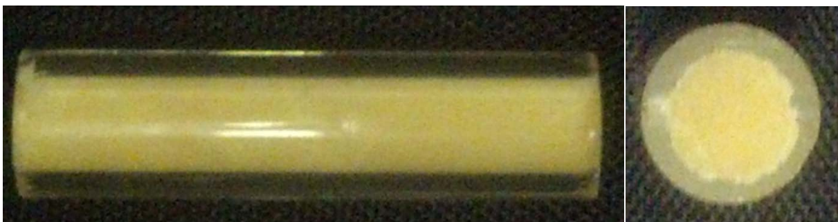
Figure 2. Pentolite cast into glass tube.
