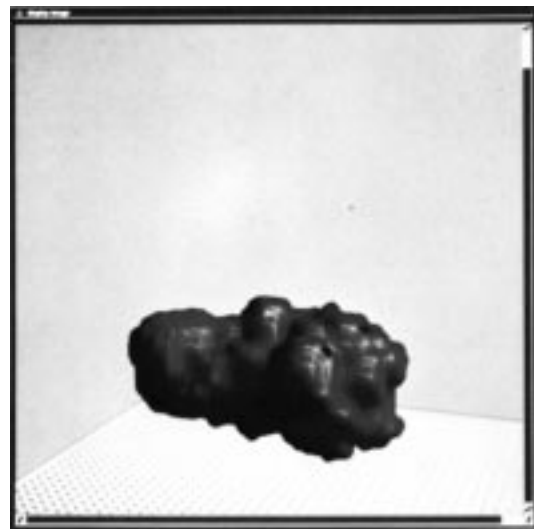
Fig. 9. The ROV as reconstructed from four passes after registration. Voxel size is 8 cm.
