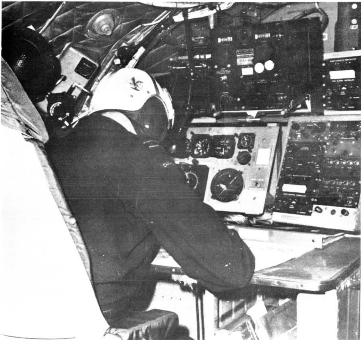
Figure 3. The lamp obscures displays and controls at the turbine navigator's station.
