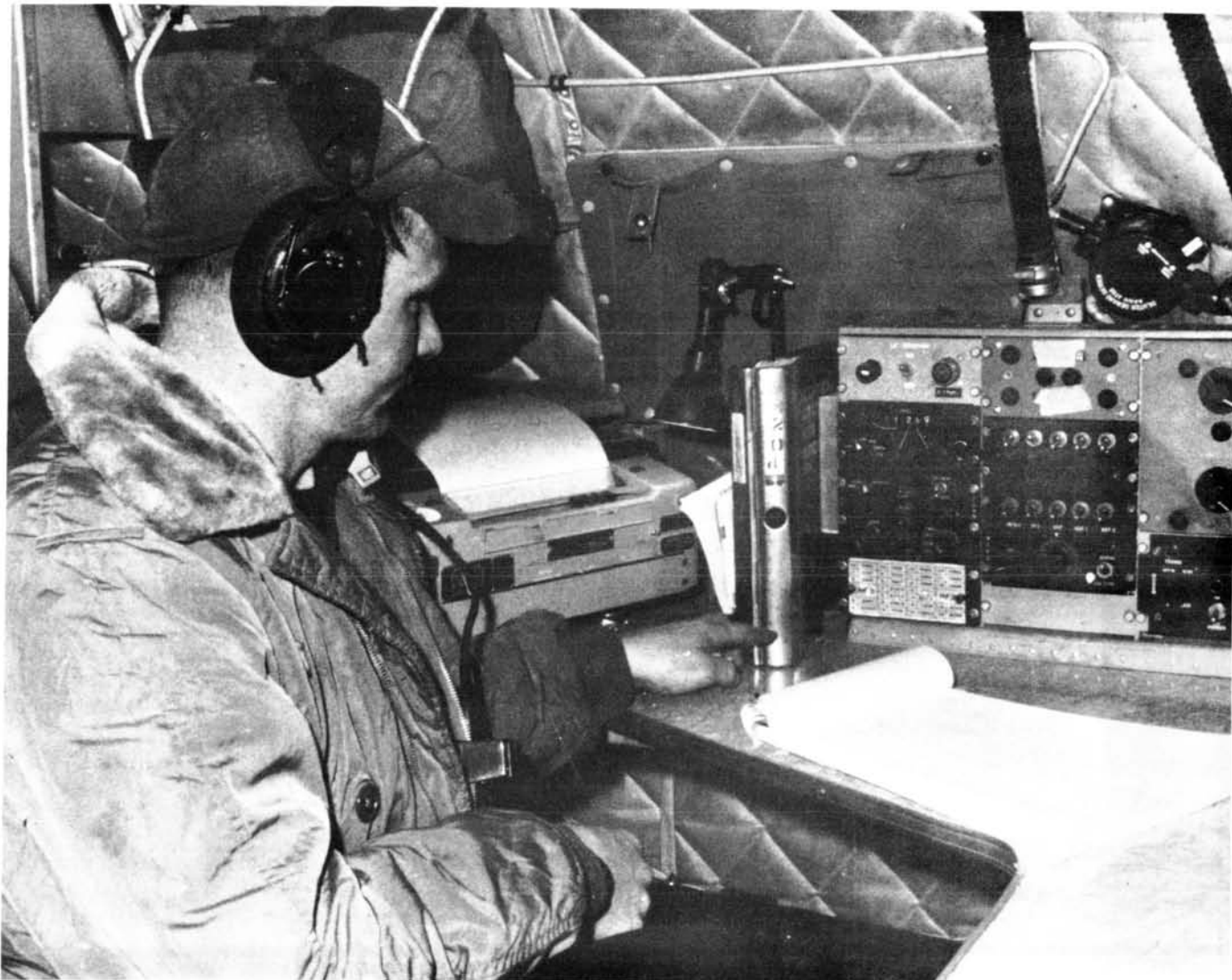
Figure 5. Displays and controls extend beyond easy reach at the radio operator's station.
