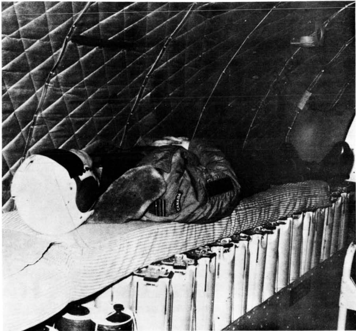
Figure 17. Additional sleeping facilities are provided by throwing spare mattresses over the aft sonobuoy storage.
