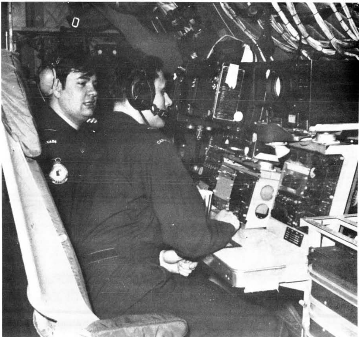
Figure 8. The main displays of the ECM operators are too high for comfortable monitoring over long periods.
