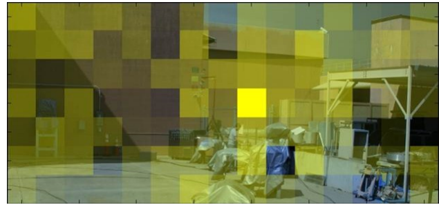
Figure 2. Coded image produced from 3-7 MeV gamma rays emitted from interrogated DU target overlaid on optical camera image. The "hot" pixel denotes the DU target location.
