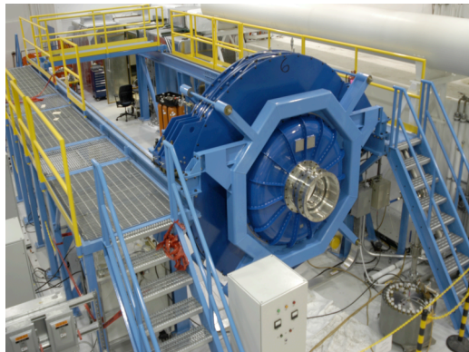
Figure 2. The MYKONOS II LTD voltage adder.
