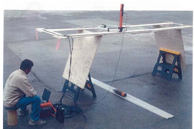
Figure 13. Test setup to evaluate a 4-meter transmitter with a small receive coil.
