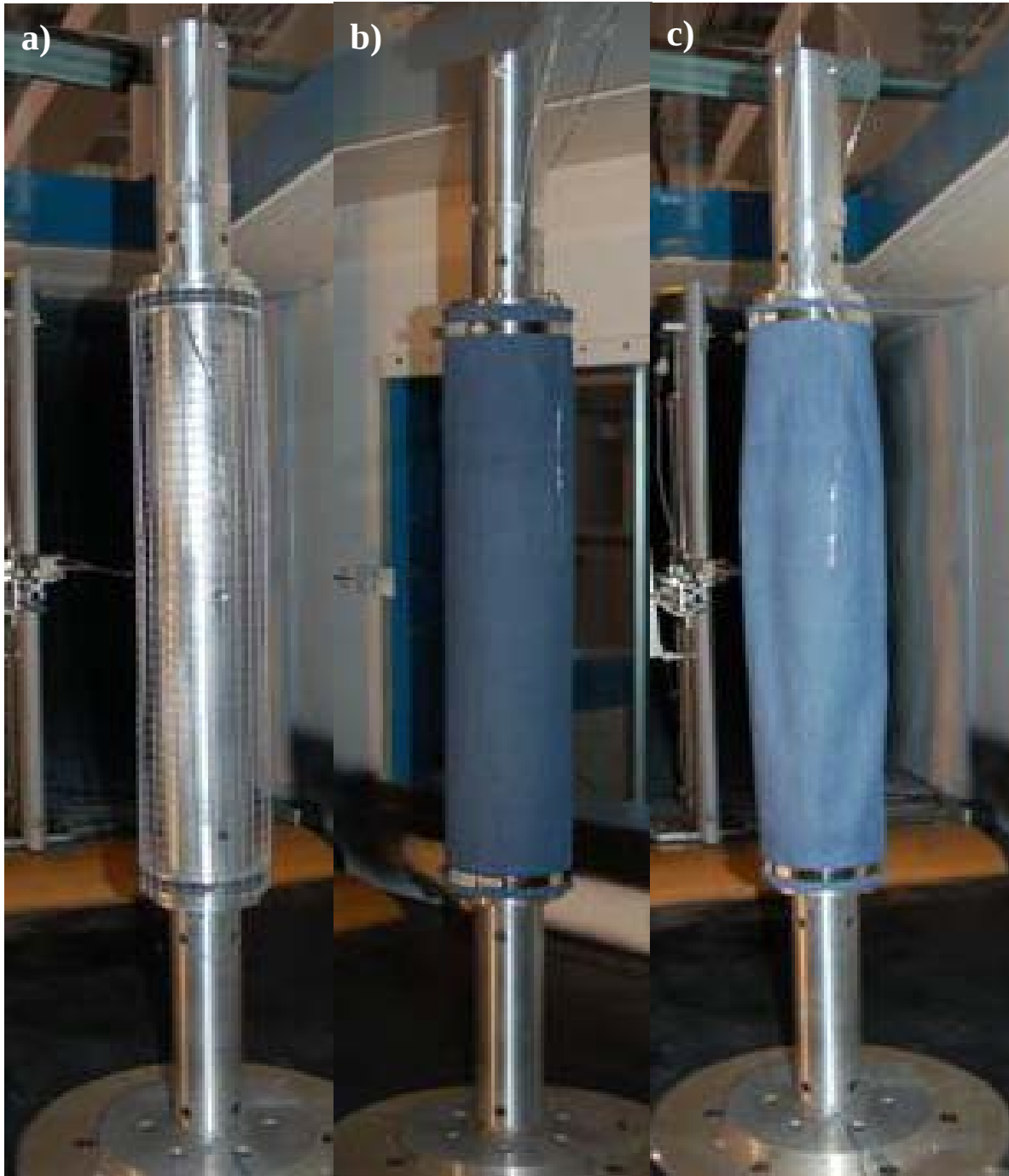
Figure A-25: Sleeve Component Fixture: a) Support Screen, b) with Installed Sleeve over the Support Screen, and c) with Installed Sleeve without Support Screen
