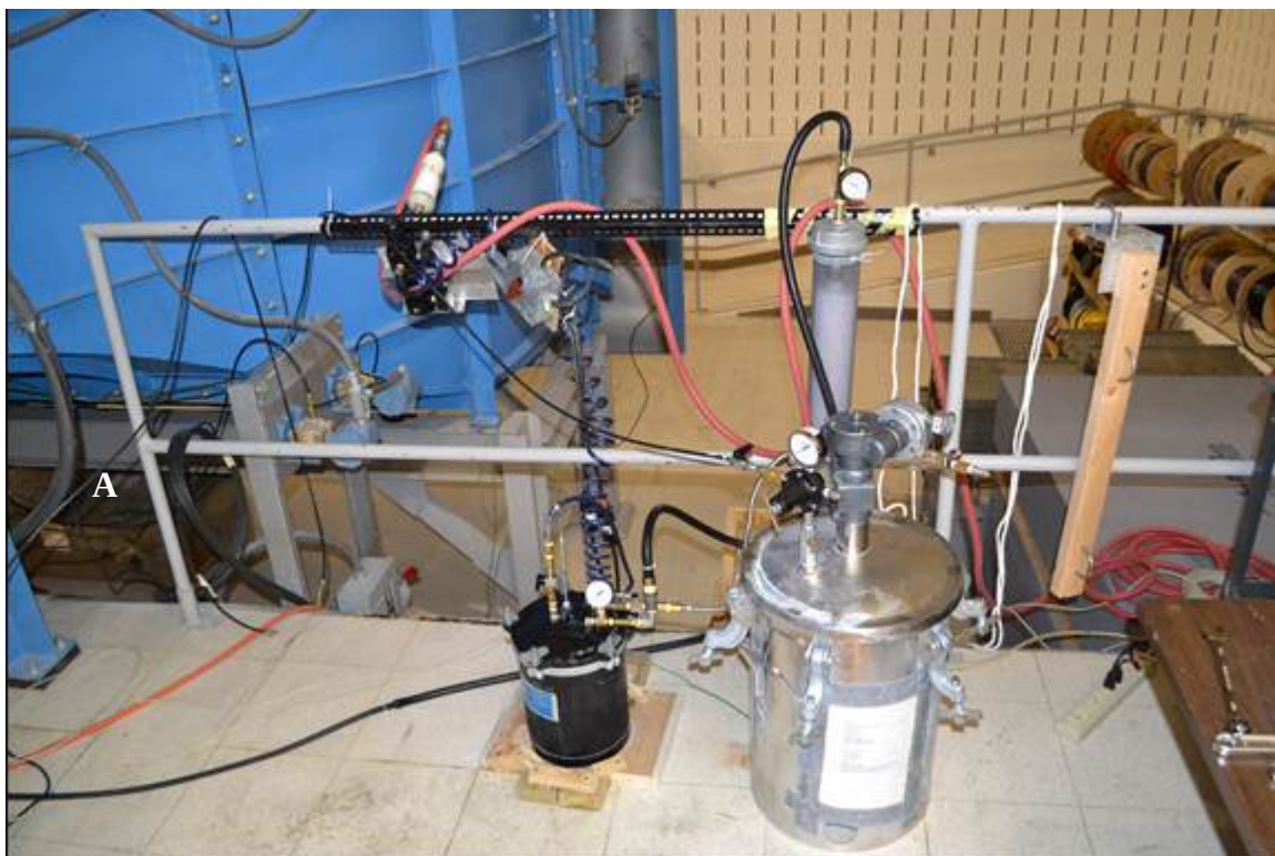
Figure A-7: DOS Dissemination System – Wind Tunnel Swatch Testing
