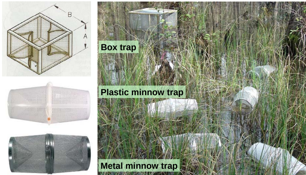
Fig. 4. Three trap types used in methods comparison study.
