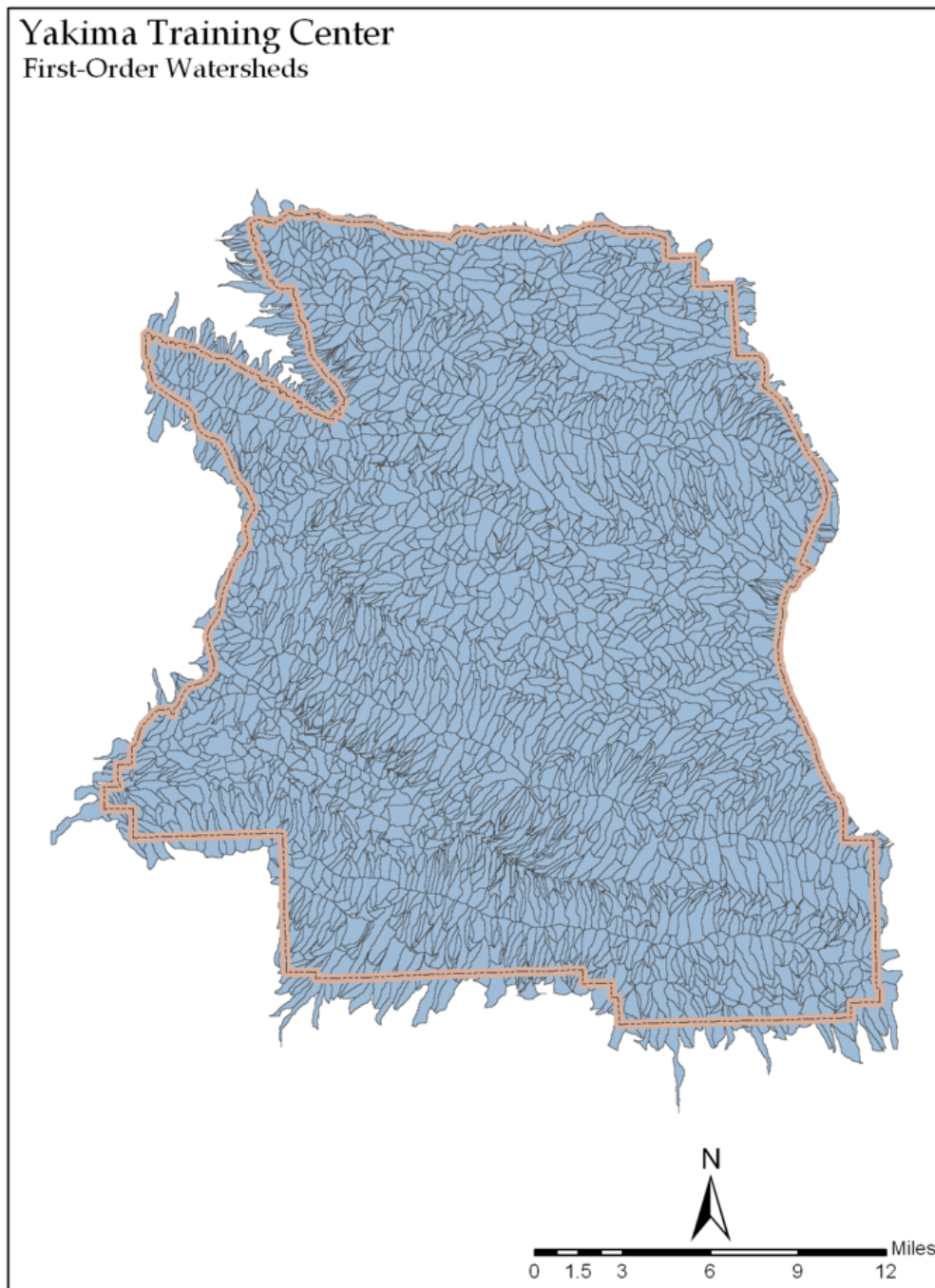
Figure 26. A total of 3,469 first-order subbasins were developed as a base for multi-scale sediment yield analysis.
