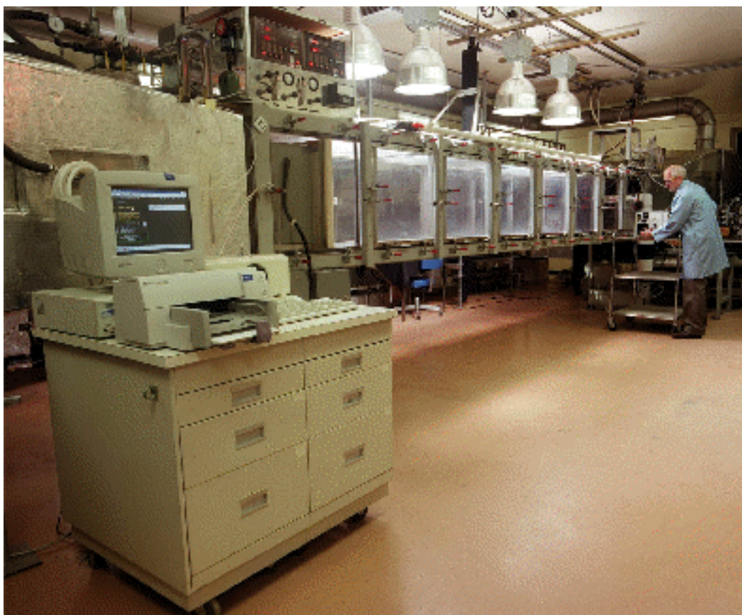
Figure 2. Environmentally Controlled Wind Tunnel at the Aerosol Research Laboratory at Pacific Northwest National Laboratory. This System Was Used to Provide Fog Oil Exposures in Typical Wind Conditions that are Optimal for Effective Obscuration.
