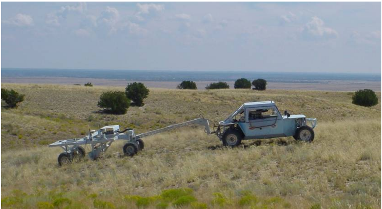
Figure 5. Ground-based magnetometer system used at the Pueblo WAA site. Magnetometer sensors are located along the structural framing mounted below the mid-section of the trailer system.
