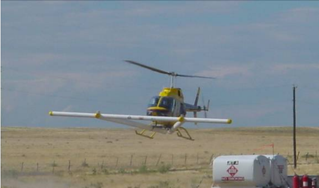
Figure 2. Helicopter-based magnetometer system used at the Pueblo WAA.
