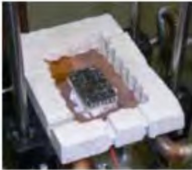
Figure 6.9 TE Module on Cold Plate with Insulator Ring in Place
