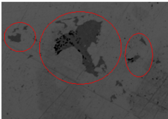
Figure 4.7 (1) SEM backscattered electron image of inclusions in as-received (not thermally cycled) refined-LAST specimen N38-10 of surface inclusions (Red ovals). As was the case for other refined-LAST specimens, no surface pits are evident on the specimen surface.
