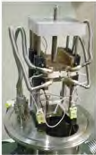
Figure 6.12 Assembled Measurement System with 2 Modules in Sandwiched Place and Stainless Steel Cooling Lines Shown
