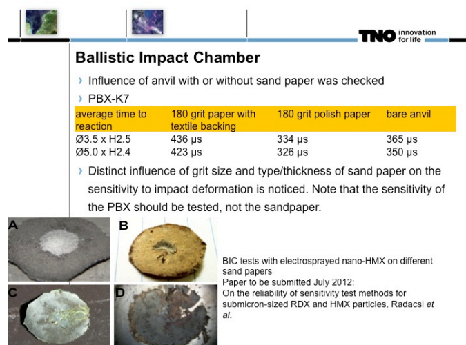
Figure 24. Effect of choice of anvil surface on BIC results.
