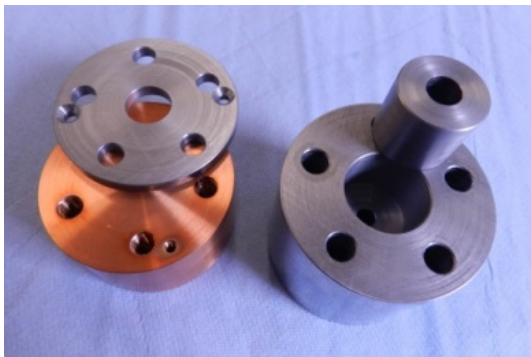
Disassembled (left) and assembled (right) Floret test set-up
