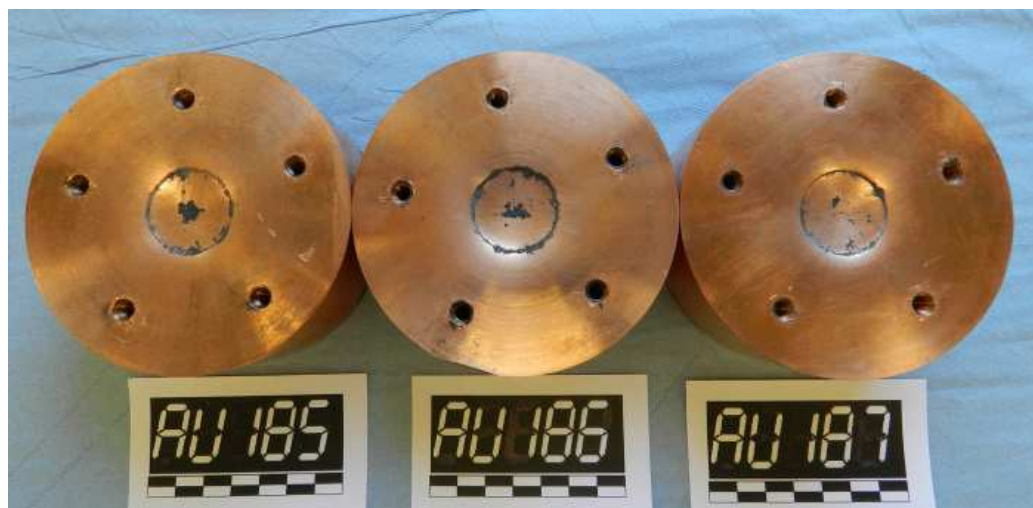
From left to right: dent profiles of RU185 (containing RDX from batch K7), RU186 (K6) and RU187 (K1).
