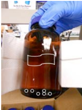
Figure 14. AC particles and a PE sampler (marked white outline to enhance visibility) in a bottle to test the sorption characteristics of AC.
