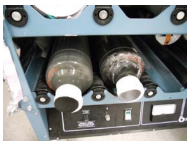
Figure 13. PE preloading sample bottles rolling for mixing.
