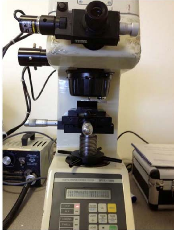
Figure 27. HVS-1000 microhardness apparatus used for the hardness measurements.
