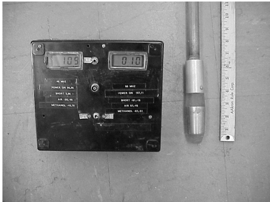
Figure 84 OSU/ESL soil probe for permittivity and conductivity measurement at 40 MHz and 60 MHz.
