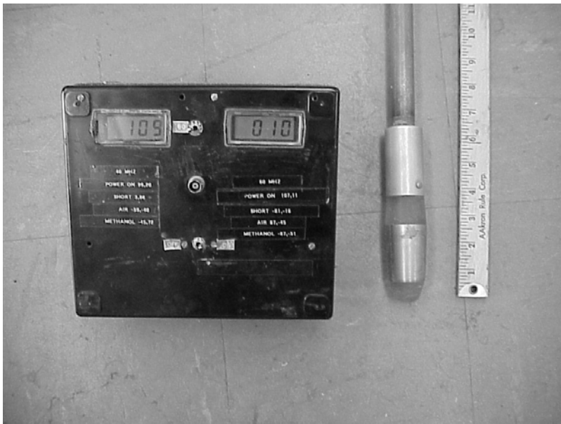
Figure 55 OSU/ESL soil probe for permittivity and conductivity measurement at 40 MHz and 60 MHz.
