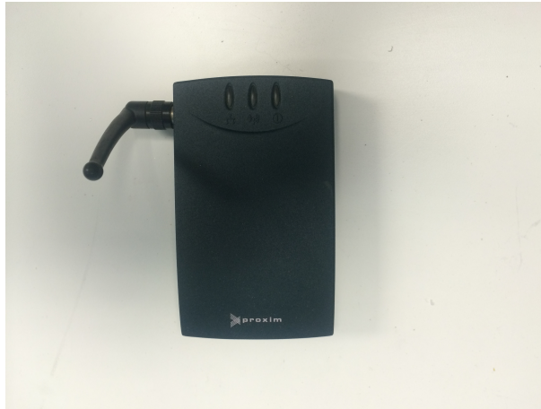
Figure 3.3: The Proxim™ modems are capable of 11540 baud and can use serial or Ethernet connections.
