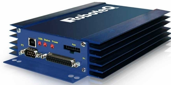
Figure 2.9: The Roboteq™ HDC2450 is a Brushed DC Motor Controller, Dual Channel, 150A, 50V, Encoder in, USB, CAN capable with on-board 32-bit microcomputer and uses Micro Basic as the language, from [8].
