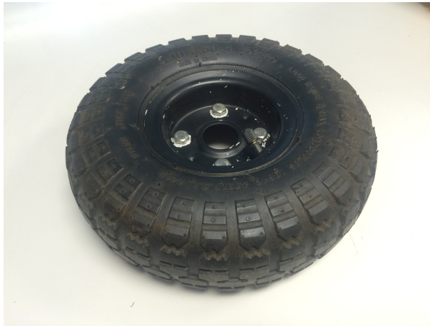
Figure 2.14: A commercial rubber nylon tube type 4.10/3.50-4 tire to test how a wider tire operates in the surf-zone environment.
