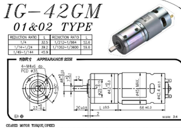
Figure 2.5: Brushed permanent magnet DC motor, variable speed and reversible, 24VDC, Reduction Ratio: 1:49, Rated Torque: 16 kgf-cm, Rated Speed: 122 RPM, and no Load Current: < 500mA, from [7].
