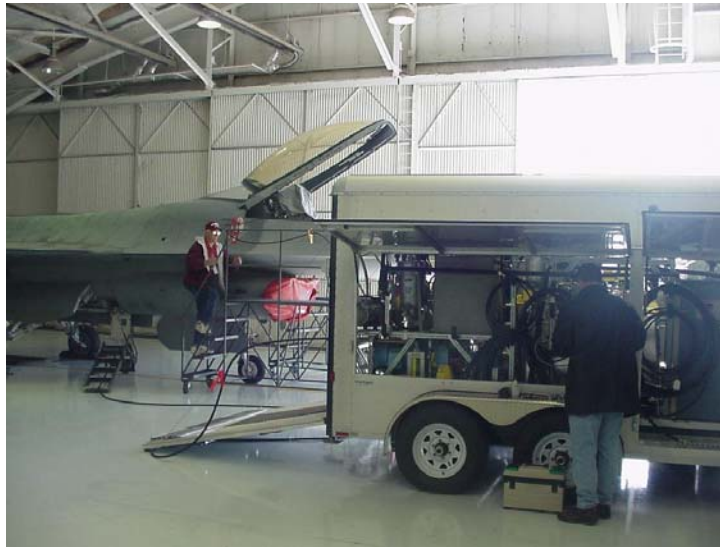
Figure 2. Versar, Inc.'s Oxygen-Line Cleaning System.
