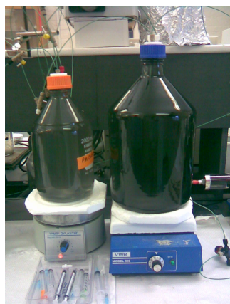
Figure 19 – PM2L (left) and PM5L (right) chemostats pictured in January 2009. Chemostats are typically covered in aluminum foil to inhibit growth of phototrophic microorganisms – the foil was removed for these photographs.
