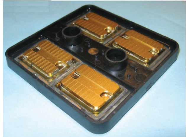
Figure 11. Four-chip Stitch SGTO module designed for voltage blocking up to 7 kV and pulse current up to 120 kA.
