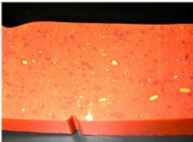
Figure 2 Cross-sectional cut of PNC/BTTN Mix IH940-97J-PNCBT-Z401
