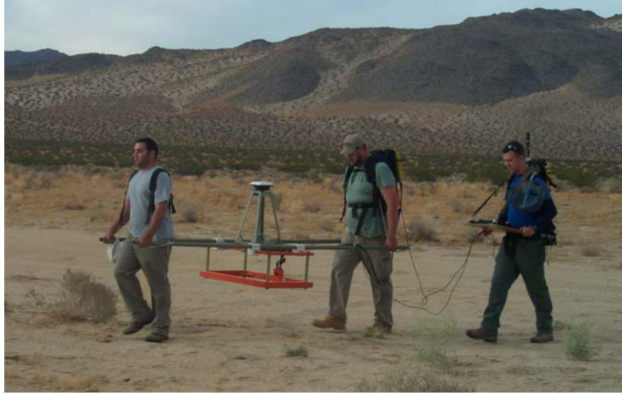
Figure 2-2 – Man-portable, litter-carried EM61 MkII sensor system as demonstrated
