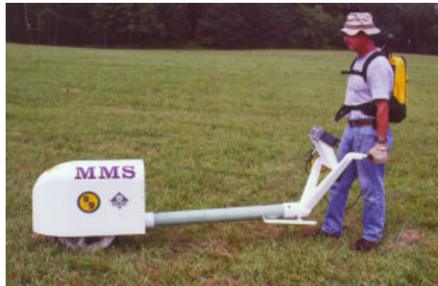
Figure 9. MMS Deployed with Protective Hood and GPS Navigation Hardware.
