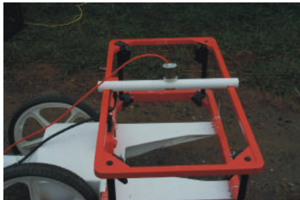
Figure 12. EMMS Deployed with the Acoustic Navigation Transponder.
