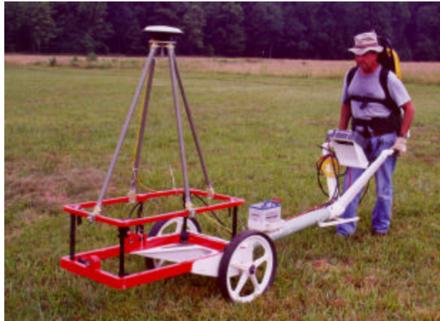
Figure 11. EMMS Shown with Digital Inclinometer and GPS Navigation Hardware.
