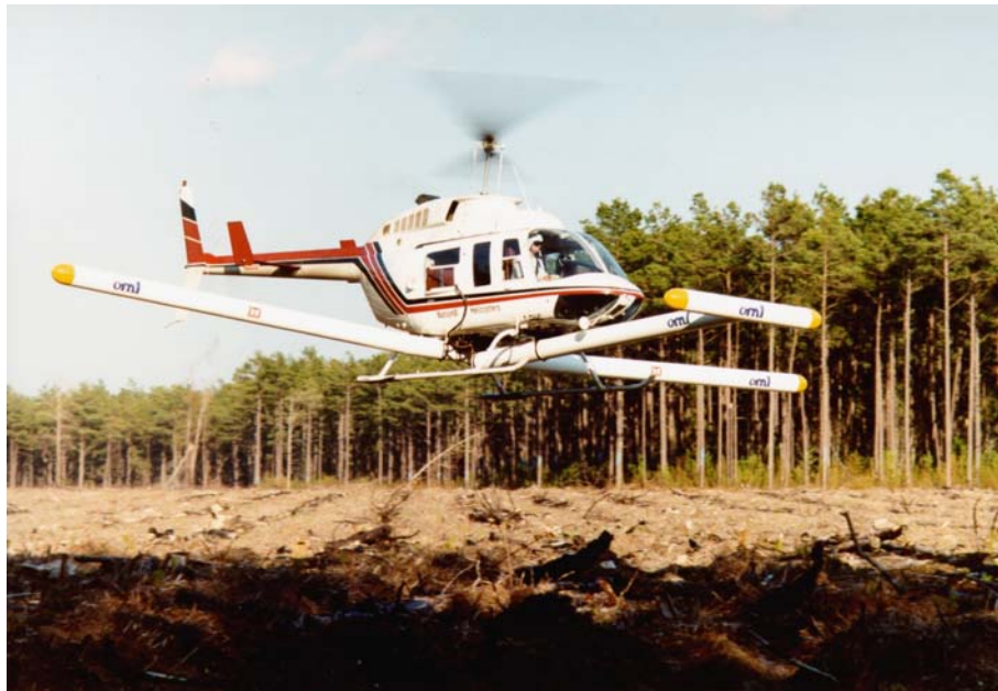
Figure 2. ORAGS-Hammerhead Airborne Magnetometer Platform at Shumaker Naval Ammunition Depot and Rocket Test Range in Arkansas.
