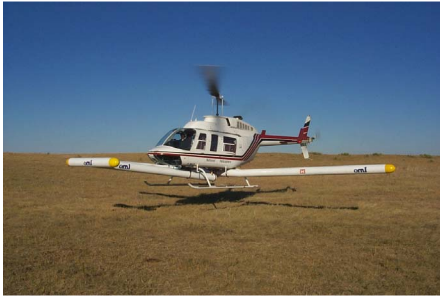
Figure 1. ORAGS-Hammerhead Airborne Magnetometer Platform at Badlands Bombing Range in South Dakota.
