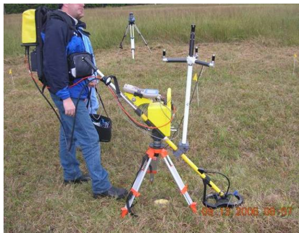
Figure 9. ArcSecond System and SAINT Mounted on EM61-HH at APG Demonstration.
