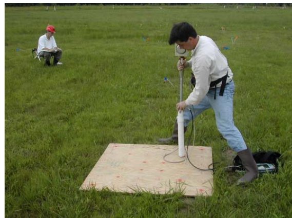
Figure 4. Static Test Grid Design with Multiple Elevations Recorded Across the Diagonals and Picture of Actual Operation Including SAINT System and PVC Standoff.
