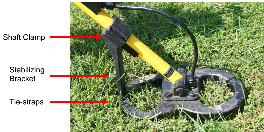
Figure 7. Hinge Locking Mechanism for EM61-HH.
