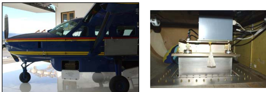
Figure 1. The C208 Fixed-Wing Platform Houses the Orthophotography and LiDAR Sensors for Concurrent Data Collection.
