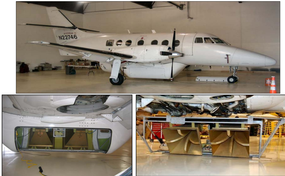
Figure 1. The Sky Research J31 Aircraft Was Used for All Aviation Activities for SAR Data Collection. (The Equipment Pod [lower-left] Houses the Bi-Static Horns Antenna [right].)
