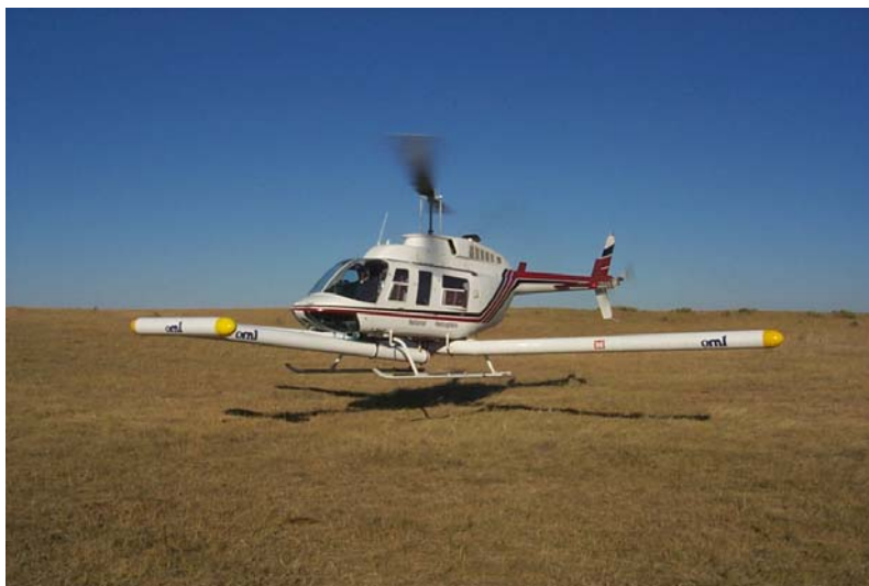
Figure 4. ORAGS-Hammerhead Airborne Magnetometer System Used at BBR in 2000.
