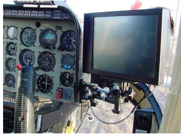
Figure 2. The Navigation Guidance Display Is Mounted on the Starboard Side of the Cockpit for the Pilot's Use During Surveys.
