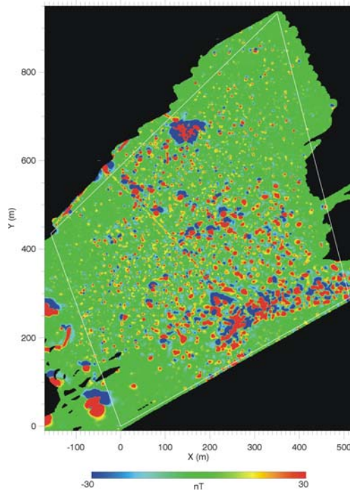
Figure 15. Magnetic Anomaly Image (interpolated) of the Active Recovery Field. (Note the cluster of surface ordnance at the top center, stockpiles of materials along the road, and the extended concentration of magnetic returns offshore.)
