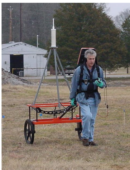
Figure 10. Ranger Mobile Radio Setup Mounted on EM61
