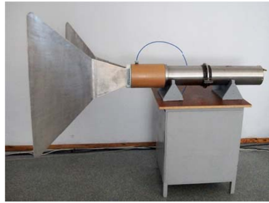
Figure 3. General view of HPM source with a field pattern converter integrated in the TEM-horn antenna
