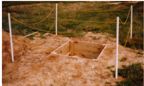
Figure 7. The CBD test pit used for shallow tests of smaller ordnance items
