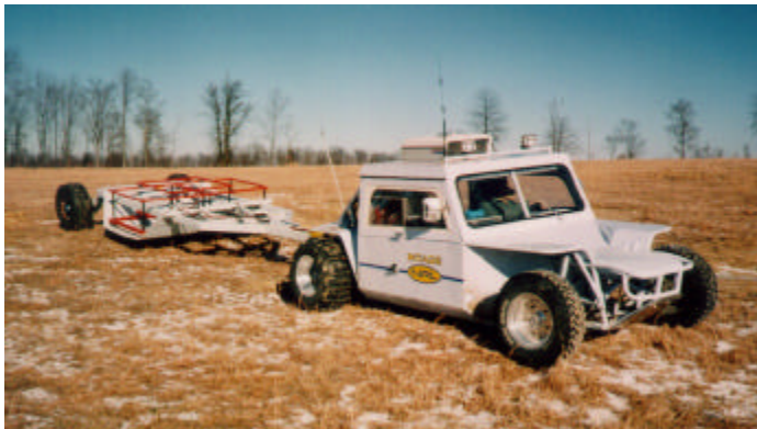
Figure 2. The MTADS deployed with the EM sensor array
