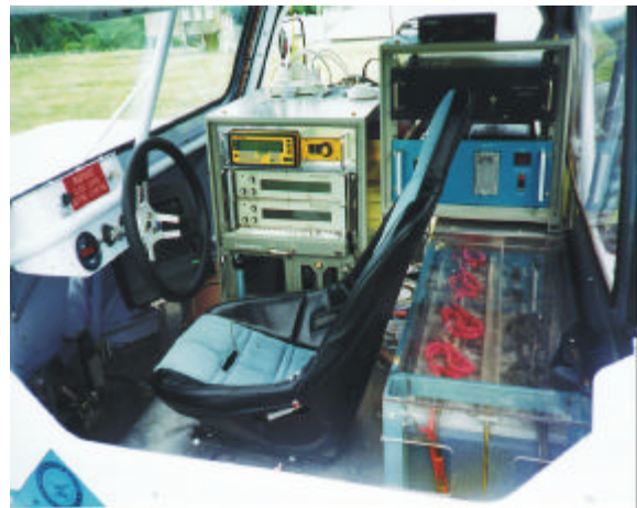
Figure 5. Layout of the MTADS Tow Vehicle showing the data acquisition and survey guidance electronics
