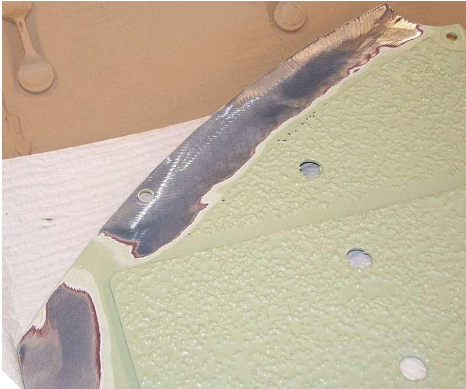
Figure 5.34: Re-Man Parts after Pretreatment of Selected Test Areas (Top) And after Primer and Top-Coat Application (Bottom)
