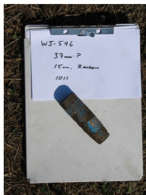
Figure 5: Photos of typical small munitions seed items used at the West Jefferson UXO Test Grid. (top left) 20mm projectile, bottom left 20mm-sized frag, (top right) 37mm projectile without rotating band, (bottom right) 37mm projectile with rotating band.
