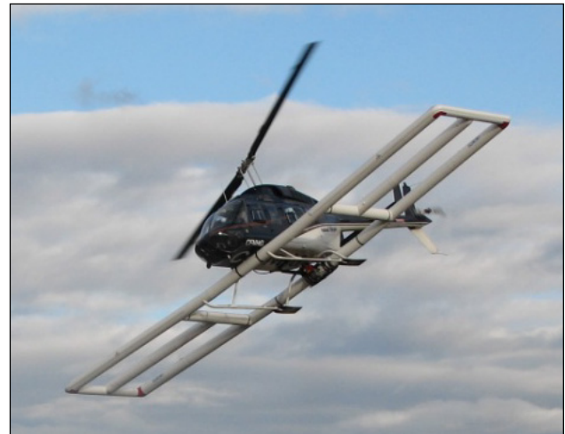
Figure 1: (a-left) Theoretical model of primary and secondary electromagnetic fields. (b-right) Photo of Battelle airborne TEM-8 system.
