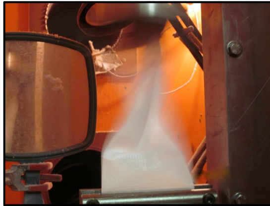
Figure 1. ILPS fabric sample during Gelbo flex testing at -40^{\circ}\text{C} . Note that the extreme twisting caused multiple folds but that these did not propagate cracks, tears, or deformities.
