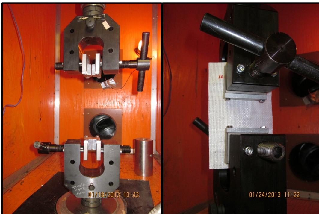
Figure 3. Aluminum adapter plates fabricated to accommodate modified (1 × 1 in.) MTS grips (left) to meet ASTM D751 specifications for tensile tests (ASTM 2011b). Sample secure in modified grip assembly and ready for testing (right).
