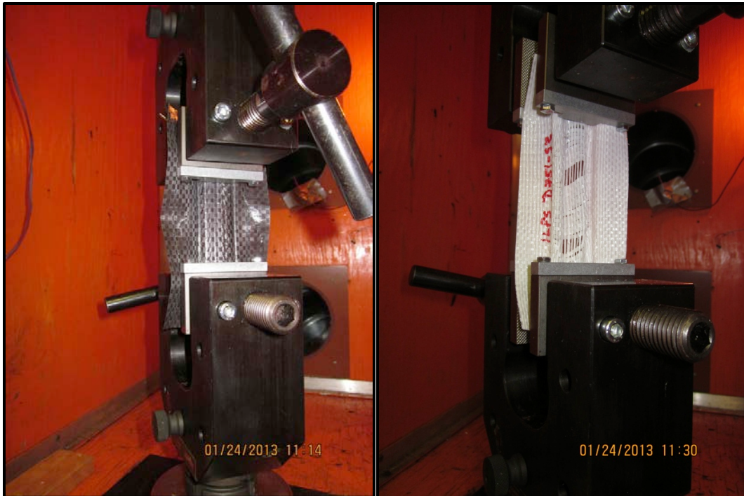
Figure 4. ILPS black protective shell fabric (left) and white structural liner fabric (right) under load during ASTM D751 (ASTM 2011b) tensile tests. Note the use of modified clamp assemblies to meet the 1 × 1 in. grip requirement.
