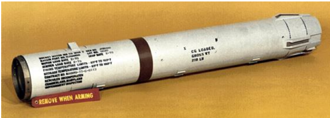
Figure 17. Mk 58 Solid Rocket Motor for NSSM 35
