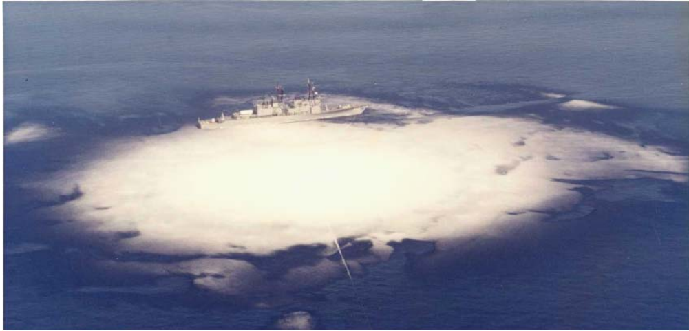
Figure 13. Photograph of Upper Surface of Bulk Cavitation, from [11]
