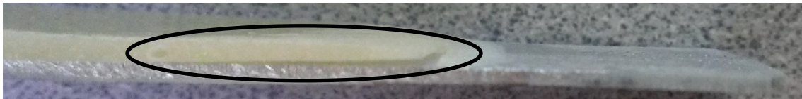
Figure 9. Delamination at the end of sample 4
