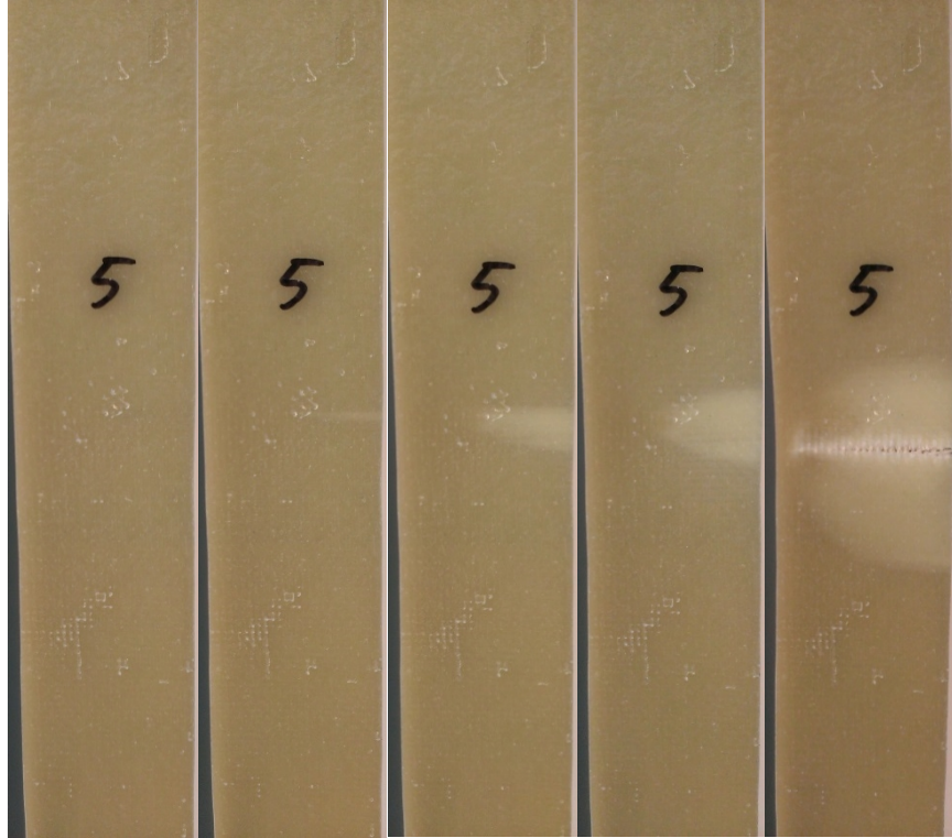
Figure 10. Delamination of sample 5 as loading is increased (left to right)
