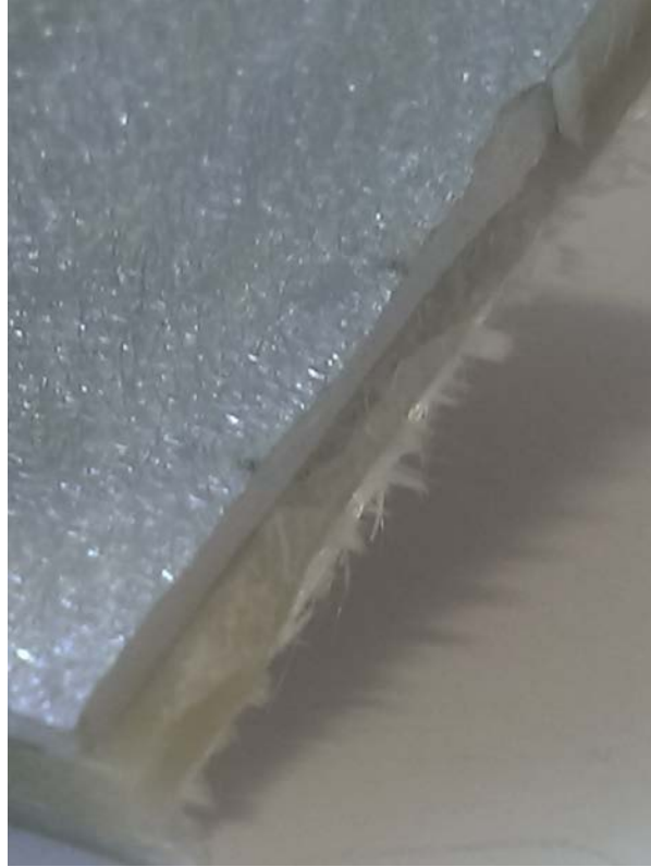
Figure 25. Cracked edge of sample 2 showing brittle fracture surface
