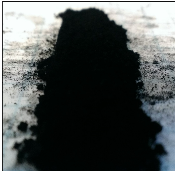
Figure 1. CNTs formed in a line two inches in length (top to bottom)
