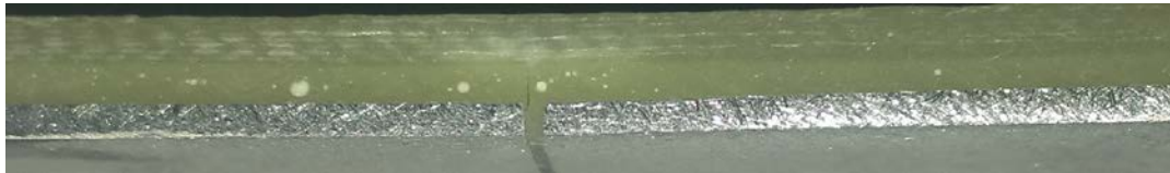
Figure 23. Sample 4 showing no delamination between layers or aluminum
