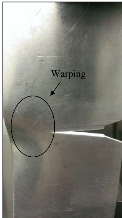
Figure 34. Bare aluminum sample with 3-inch width, warping can be seen on left side
