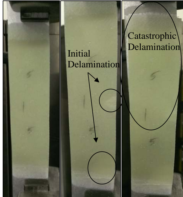
Figure 36. Eight inch samples, before testing (left), initial delamination (middle), final catastrophic delamination (right)
