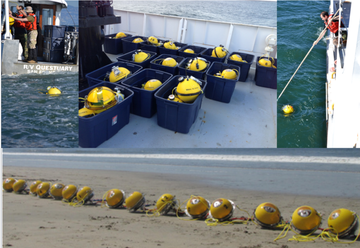
Figure 15. Three different types of Wave Resolving Drifters (WRD). The WRD-A deployed from the R/V QUESTUARY (top left). The mix of WRD A-B-J on the deck of the R/V POINT SUR (top center). The WRD boat hook recovery (top right). The more advanced WRD-J (bottom).
