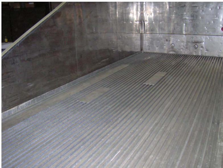
Figure 12. Interior view of the completed lysimeter demonstrating the ridged bottom to facilitate flow of the leachate from the amended ballistic sand.
