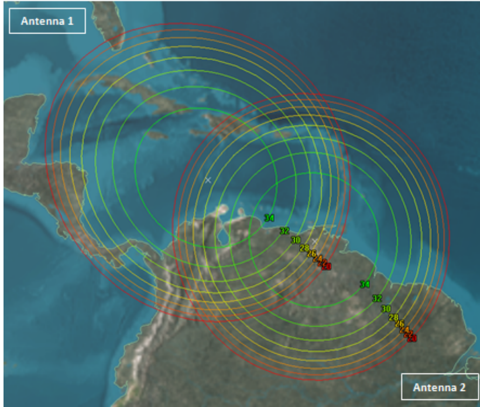
Figure 14. Two Adjacent 25 GHz Antenna Patterns Down to 20 dB ( G_1 and G_2 ).
