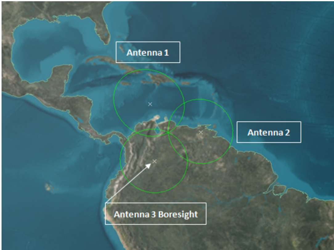
Figure 8. Three Slightly Overlapping 2 Degree Beamwidth Antenna Patterns.
