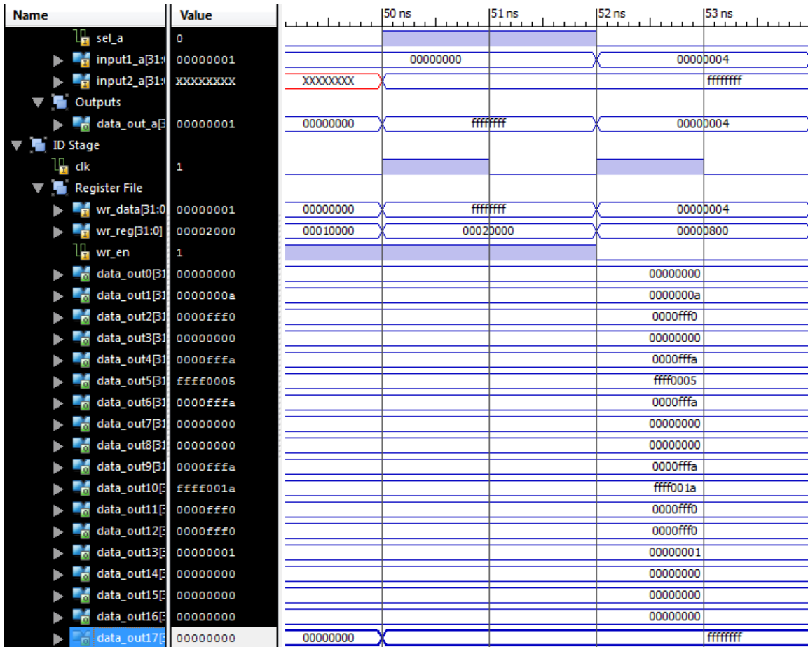
Figure 40. WB stage outputs for the load word and store word instructions.
