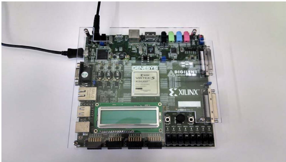
Figure 10. Digilent Genesys Virtex-5 development board.
