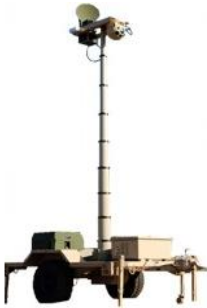
Figure 14. Trailer-mounted GBOSS system configured for operation 69
