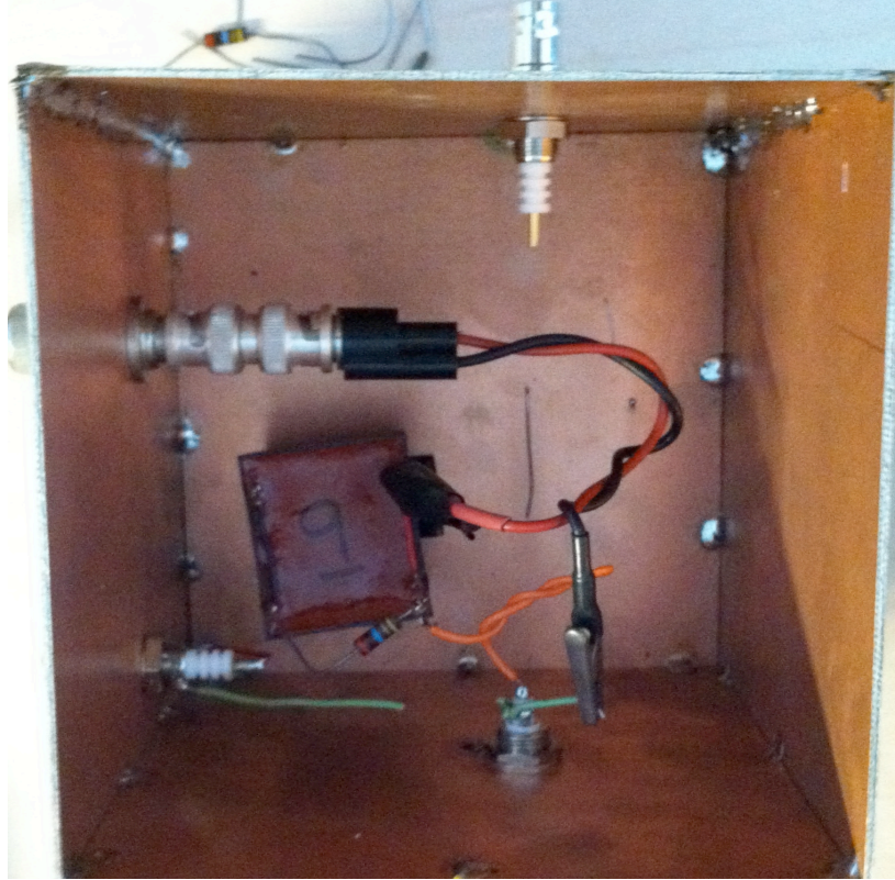
Figure 13. Air connection method used to prevent excessive noise and signal distortion.
