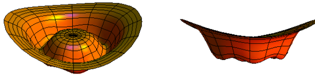
Figure 7.4: Potential well for the case of a fundamentally symmetric system that has been perturbed by the switch beam. There are still two global minima but now they have been rotated by \pi/3 relative to Fig. 7.3. The parameters used in Eq. (7.3) to generate this plot are p = 0 , r = 1 , h = 0.1 , and s = 0.1 .
