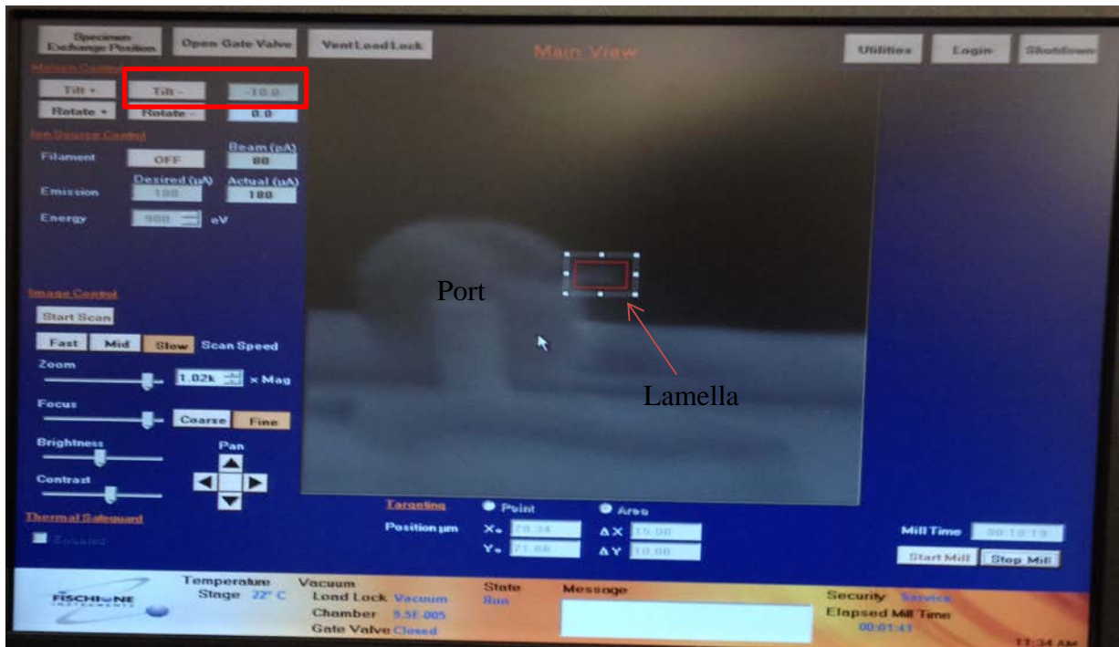
Figure 21. NanoMill control screen depicting the -10^{\circ} tilt angle and underside of the port.
