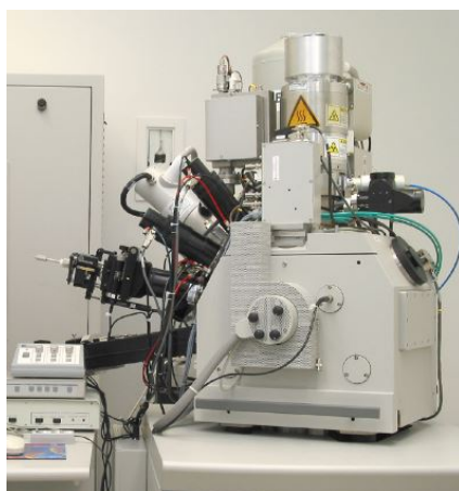
Figure 7. FIB with OmniProbe on the left with the SEM stack on the top.
