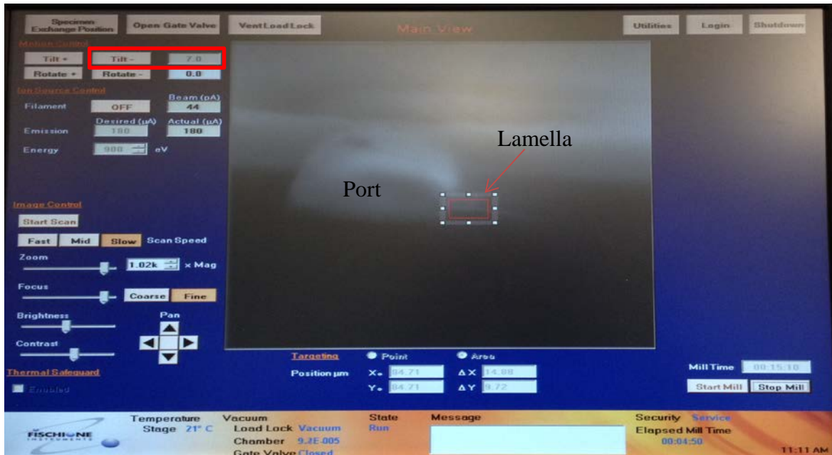
Figure 20. NanoMill control screen showing parameters for the milling process and monitor screen.
