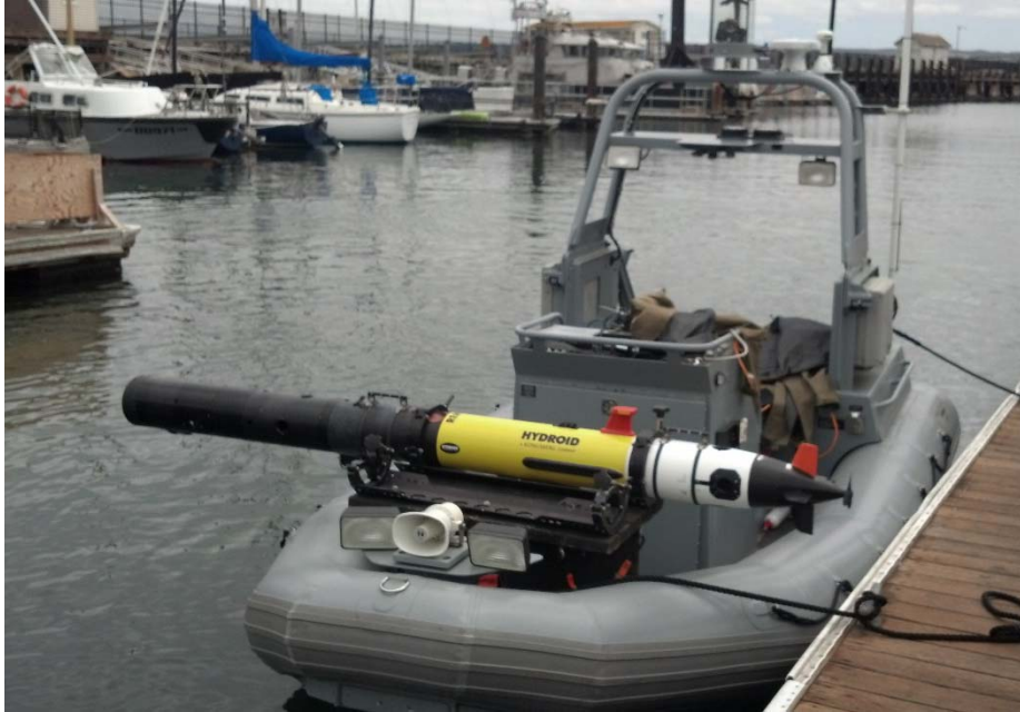
Figure 1. REMUS 100 AUV onboard CAVR's SeaFox surface vessel
