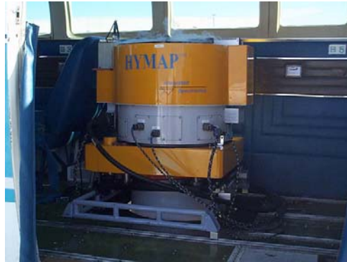
Figure 2. The HyMap instrument mounted in a twin-engine light aircraft with gyro-stabilized mount and looking through a standard aerial photo port.
