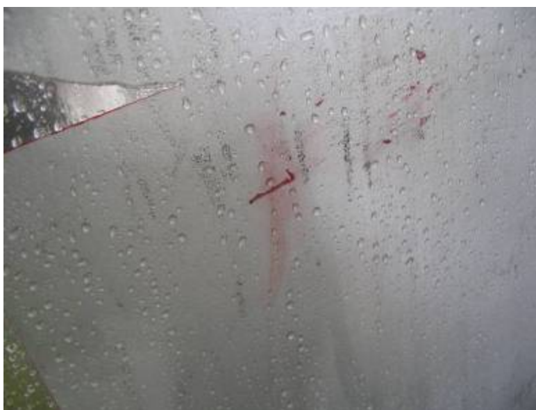
Figure D19B. Glue Colored by VCPI Solution
