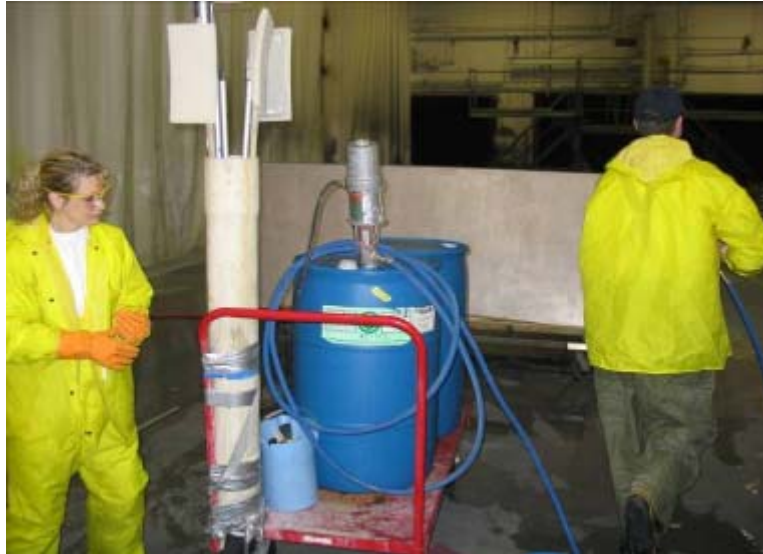
Figure D3. ReGel® Being Sprayed on Stripped Panels
