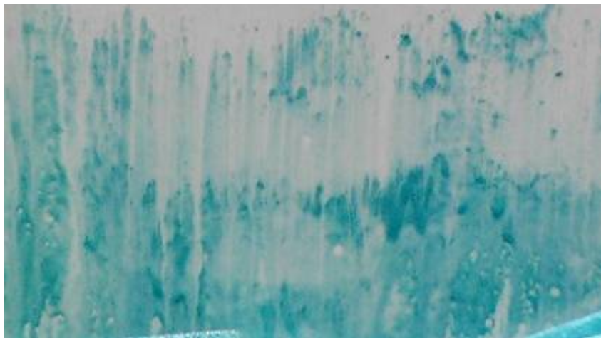
Figure 11. Post-rinse VCPI Labeling of Soluble Salts on Hull of USS Halyburton
