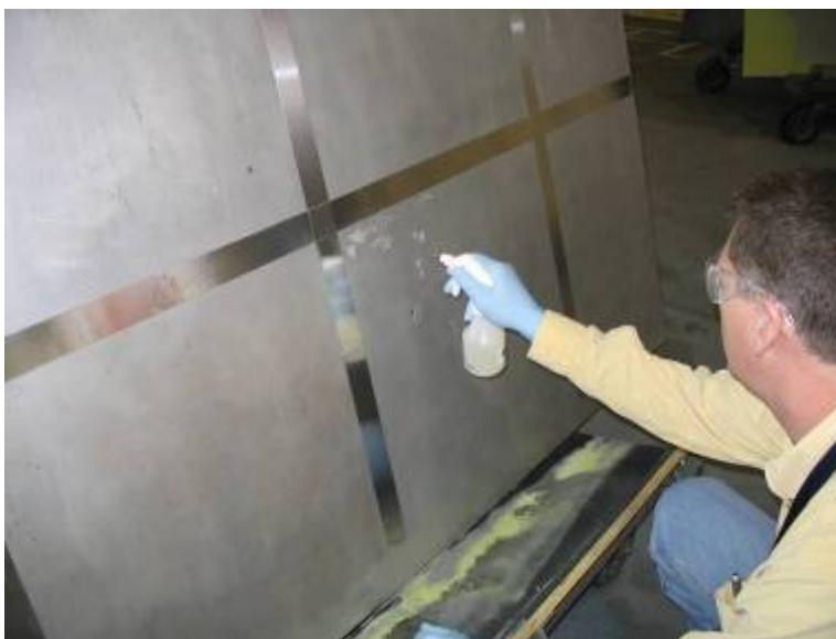
Figure D12. PreKote ® Being Sprayed onto Surface
