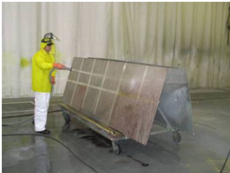
Figure D17. VCPI Solution Being Rinsed from Panel "A"
