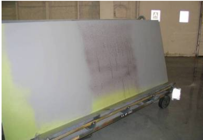
Figure D27. VCPI Solution Applied to the APC Painted Panel
