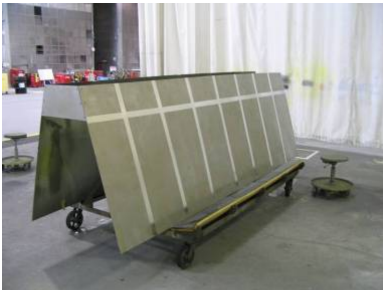
Figure D10. “B” Panel (Rear) Divided Into Eight Vertical Sections
