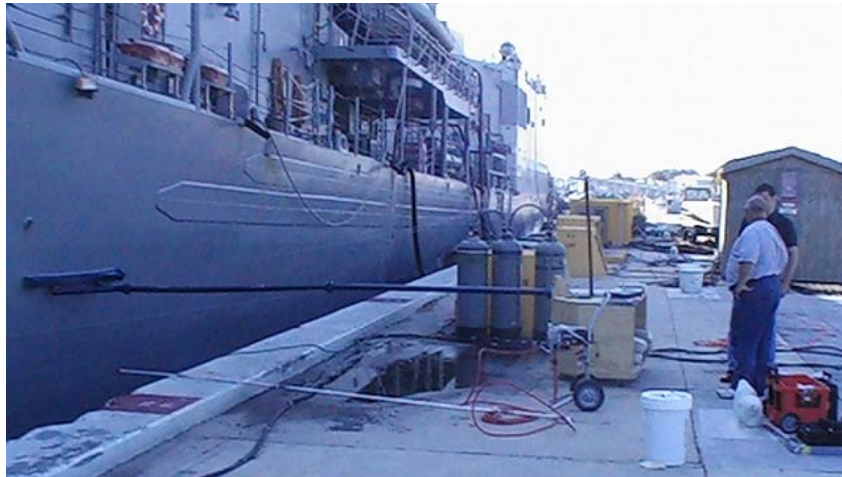
Figure 10. VCPI and Rinse Water Containment Equipment on Hull Surface
