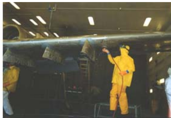
Figure A11. Application of PreKote Surface Pretreatment
