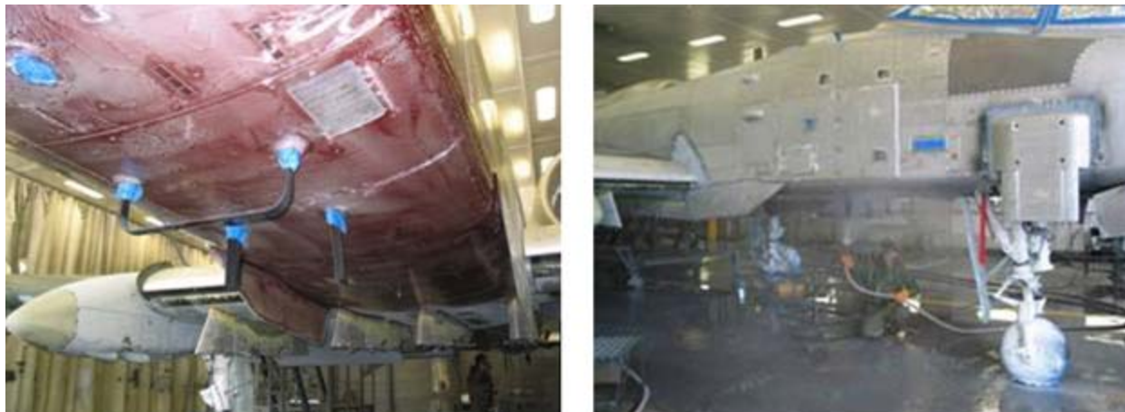
Figure 6. Application and Removal of VCPI Test Solution to Lower Fuselage of A-10 Aircraft at Hill AFB, UT.
