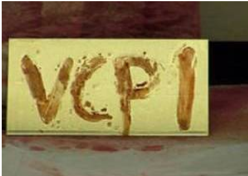
Figure 3. Visually-indicated Contamination after Solvent Rinsing
