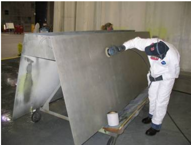
Figure D6. Surface Power Scrubbed Using Pneumatic Tools
